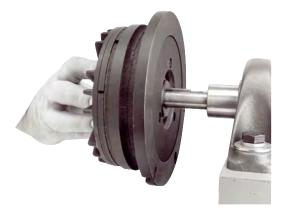
5. Install the optional Warner Electric torque arm or the customer furnished pin. The arm must be strong enough to withstand the brake's full torque capacity, and should be affixed to the machine frame, and to the brake tangent to its circumference in the notched attachment point on the back plate. It must also be flexible enough to compensate normal shaft and bearing runout without causing binding or side loading to the brake.
