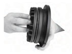
4. Slide the brake onto its shaft over its key. If the brake is to be operated in a vertical position, it must be mounted with the armature fins up.
